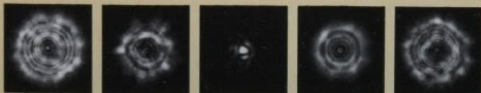
The all-too-familiar effect of atmospheric seeing. These are five freeze-frames of simulated mediocre turbulence, quality 5 on the usual scale of 1 to 10 (aberrations about \frac{1}{2} wave peak to peak). The aperture's diameter is 20 percent obstructed.
