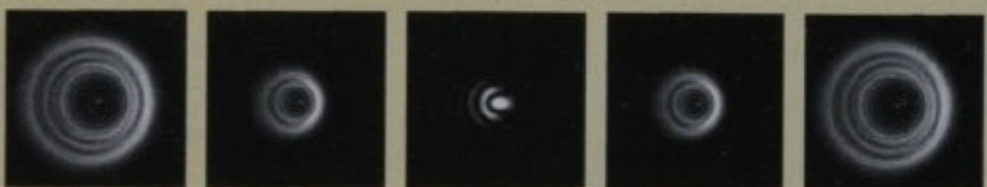
The sign of poor collimation. Even though these patterns are asymmetric, they appear similar on both sides of focus. The lower a telescope's f /ratio, the more crucial collimation becomes; this is what a mere 6 arc minutes of misalignment looks like in a 10-inch f/4.5 reflector. The optical axis is to the right of the star image.
