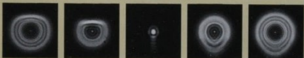
The effect of warm air ducting along the inside upper wall of a tilted telescope tube, a common but temporary thermal problem.
