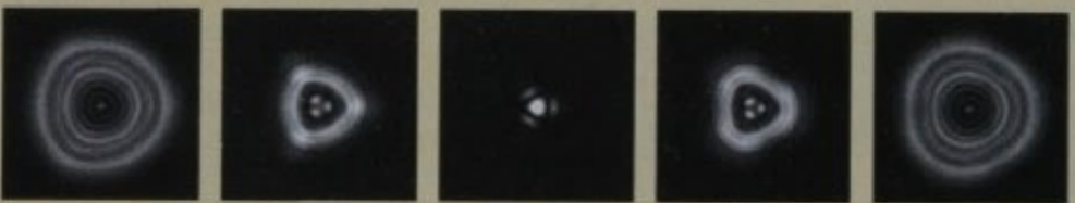
A triangular deformity is a sign that the mirror is probably being squeezed in its cell. Loosen the mirror clips slightly to relieve the bending of the glass. Check for undue sideways stresses too.
